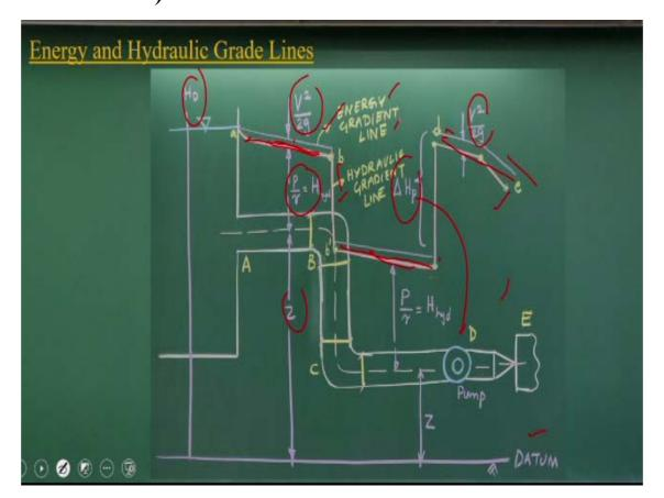
Again I am repeating it this energy gradient line and hydraulic gradient line what we discussed just after the Bernoulli's equations. Now let us I have the reservoir, okay. This is the datum. From the reservoirs I have the pipe systems okay and there is a pumping system. So you can draw hydraulic gradient line, also we can draw the energy gradient line.
