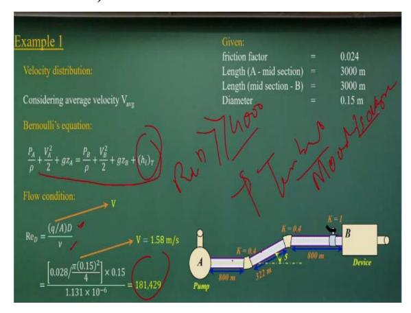
So first I say that we should have a modified Bernoulli's equations with the head loss components okay, modified Bernoulli's equations with the head loss components. First what you do it we should compute the flow Reynolds numbers okay. So here we are substituting with in terms of diameters and we are computing the flow Reynolds numbers which is coming out to be so large numbers okay.
