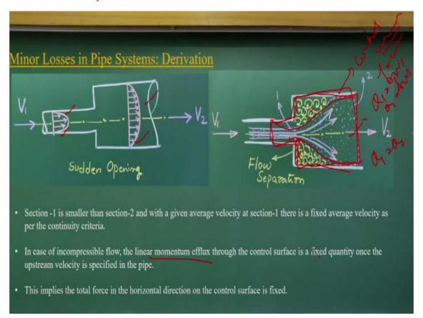
Let us come for derivations of energy losses and the pressure and velocity distributions of having a systems where two pipes we are enlarging it from the smaller diameter to bigger diameters. If you have that conditions and you can draw the velocity distributions. The velocity distribution it depends upon the type of the flow. If I have a laminar flow, the velocity distribution is different.
