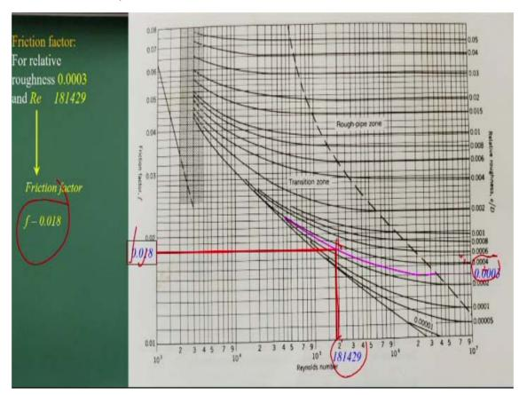
Identify this approximately which the curve will come there. You know, these Reynolds number, compute it that. Draw the lines with matching that then compute this friction factors, okay? It is very easy. Using this Moody's diagrams, you can first identify with respect to the relative which curve we should follow it. But if curve is not there exactly we can interpolate it that curve and know the Reynolds numbers, interpolate it this.
