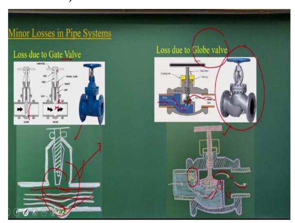
If you look it that most of the times also we have a valve to control the flow okay which is a gate valve okay, it is a gate type of systems. If you rotate it this valve closes the waters okay. And it can have a total open or half closed and all these conditions to regulate the flow to regulate the flow we have a these systems. Now if you look it if I am to draw the streamlines, how it happens it.
