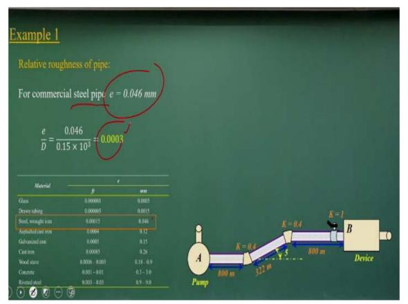
So this is a commercial steel pipe. So roughness value is given to here. The relative roughness value is know it. And once you know the relative roughness value, we are getting it this value and we are computing the relative roughness values.
