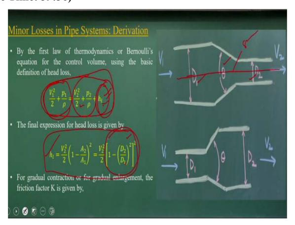
Now I will applying Bernoulli's equations along the straight line, okay I am just applying the Bernoulli's equation along the straight line. When you apply the Bernoulli's equations, this line is horizontal. This streamline is horizontal, so you do not have a z components. You have pressure head component and the velocity head component. That is what you equate,
